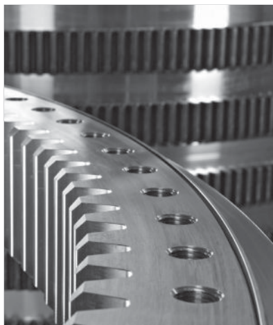
IV Schrappen Grob Coarse roughing of internal gears
