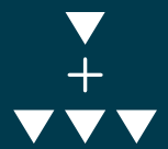
Roughing and finishing
