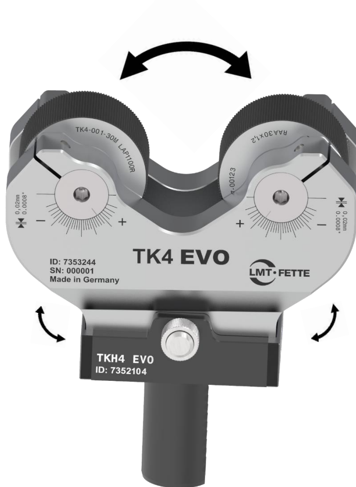
Figure 14: Checking the pendular play of the rolling head in the holder
